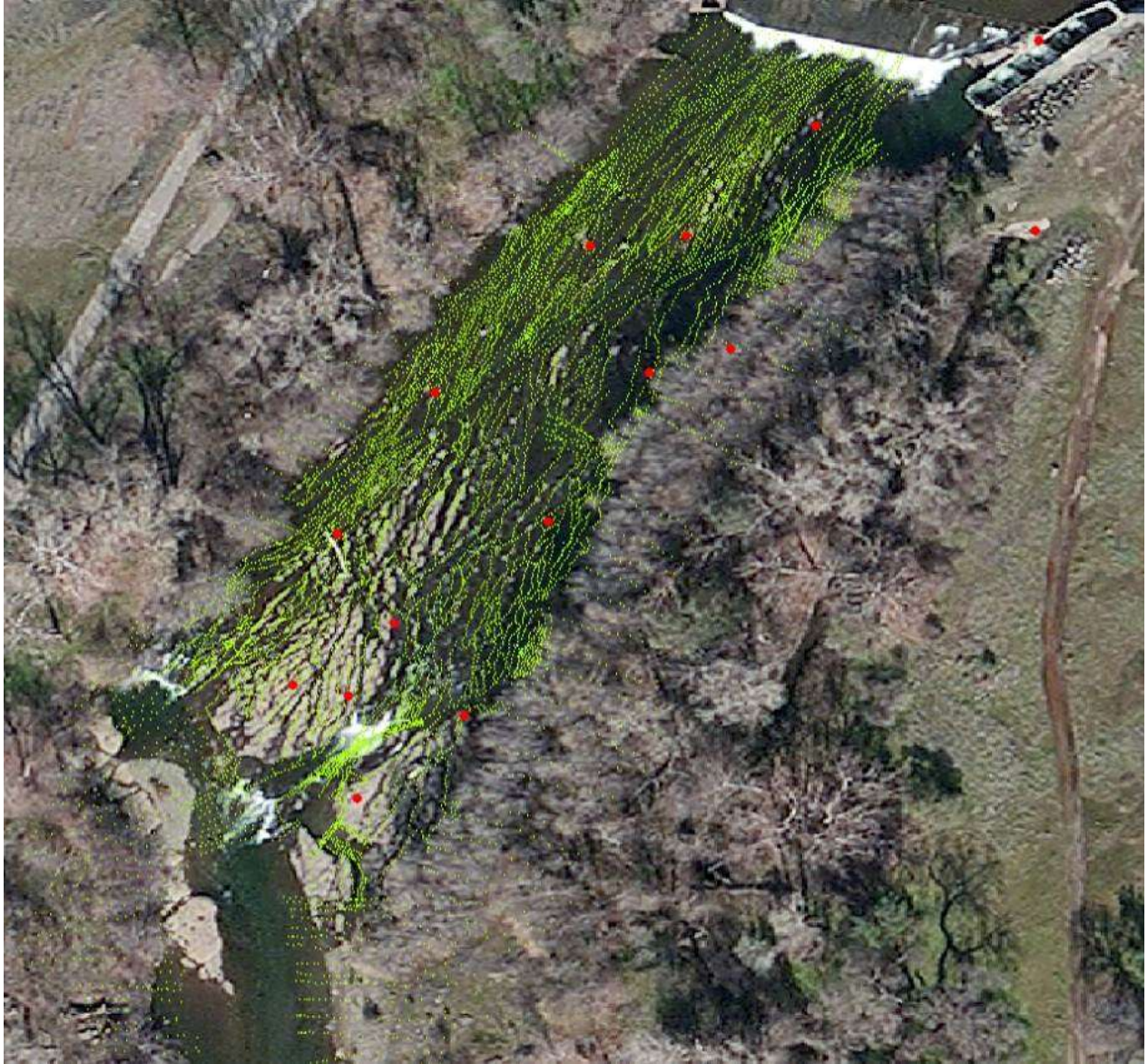
Figure 21. Data points collected with RTK GPS and total station (green dots) and control points used for terrestrial LIDAR (red points) for the Lahar site.
