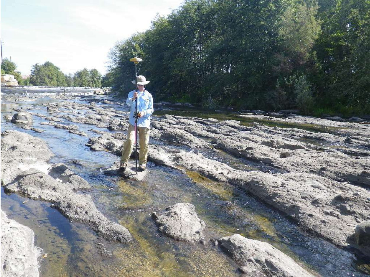
Figure 20. RTK GPS survey of Lahar Site.
