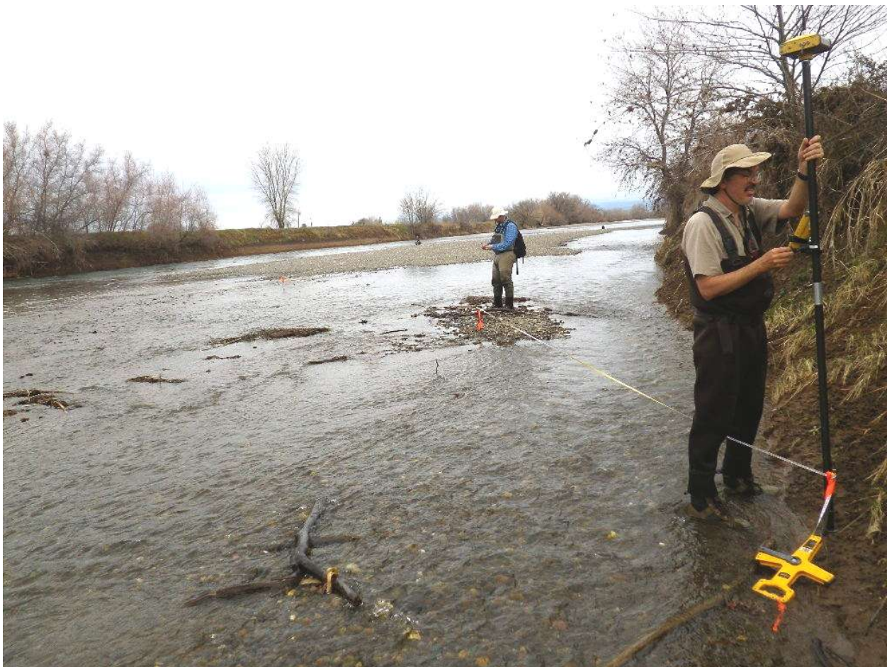
Figure 13. Critical riffle analysis transect following shallowest course from bank to bank at Riffle 97 at approximately 402 cfs.
